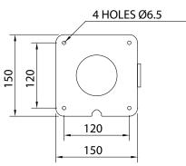
Comprising a robust Black Polycarbonate Base, and a Polycarbonate lens. Multiple units from the Series T, Series U, Series V and Series W ranges can be joined together, including the matching IAS-T Sounder and ISB-T Sounder Beacon, to provide an integrated signalling system.
