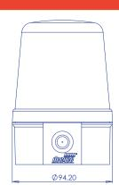
Series B is an IP66 rated enclosure, pre-moulded with drill-outs for M10 and M20 cable gland entries. The lens fits with a specially designed O-ring and tightens on a bayonet-style fitting, securing with an anti-tamper screw into a blind hole.
