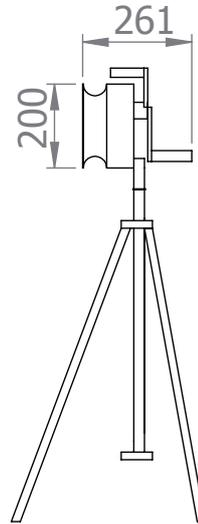
Die cast aluminium siren with tripod designed as a back-up alarm when there is a power failure or for applications where no electricity is available.
