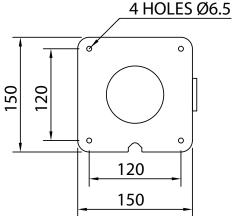
Hood assembly is fitted to the base using a gasket and three screws. Mounting to panels, walls or brackets is by four external mounting holes.
