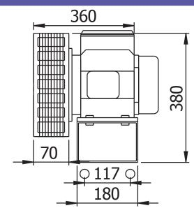
Very durable weatherproof motor driven siren manufactured from cast aluminium with high-power low-frequency output.
