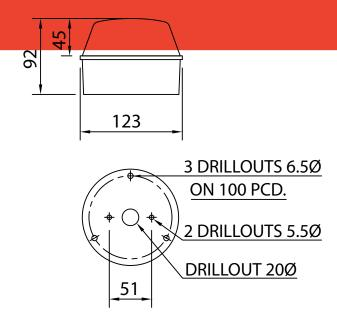
Compact xenon strobe visual warning device featuring ABS base and polycarbonate dome lens. Bases available in White (standard) or Black whilst lenses are available in Red, Amber, Green, Blue or Clear.
