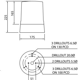
A traditional rotating mirror beacon with solid state LED light source. Extremely high light output and a very pure colour obtained from using the same colour LED as beacon lens. Red, Amber, Green, Blue, Clear colour options are available.
