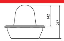
A traditional rotating mirror beacon with solid state LED light source. Extremely high light output and a very pure colour obtained from using the same colour LED as beacon lens. Red, Amber, Green, Blue, Clear colour options are available.
