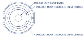
The lens fits with a specially designed O-ring and tightens on a bayonet-style fitting, securing with an anti-tamper screw into a blind hole.
