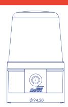
Solid-state LED beacon with revolving (simulated rotating) light effect. 360 degree 'all-round' visibility and no moving parts.
