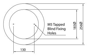
Multi-function Rotating/Pulsed/Static LED Beacon with 8 operating modes. Comprising a robust White Polycarbonate Base, and a Polycarbonate lens.
