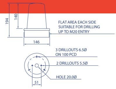
Traditional high-dome xenon strobe visual warning device featuring ABS base and polycarbonate dome lens. Bases available in White (standard), Black or Red whilst lenses are available in Red, Amber, Green, Blue or Clear.
