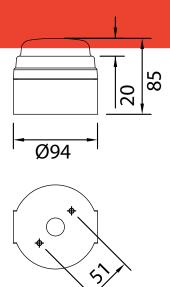
IPC/012 - Pulsed (Flashing) LED Single Green Arrow Indicator with internal jumper to select Static (Continuous) option.
