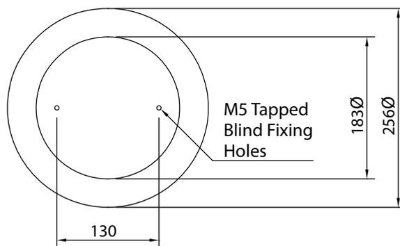
Multi-function Rotating/Pulsed/Static LED Beacon with 8 operating modes. Comprising a robust White Polycarbonate Base, and a Polycarbonate lens.
