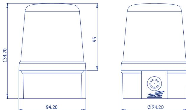
Solid-state LED beacon with revolving (simulated rotating) light effect. 360 degree 'all-round' visibility and no moving parts.
