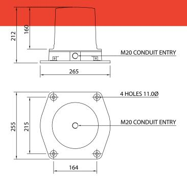
Multi-function Rotating/Pulsed/Static LED Beacon with 8 operating modes. Comprising a robust White EPC Cast Aluminium Base, and a Polycarbonate lens.
