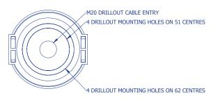
Series B is an IP66 rated enclosure, pre-moulded with drill-outs for M10 and M20 cable gland entries. The lens fits with a specially designed O-ring and tightens on a bayonet-style fitting, securing with an anti-tamper screw into a blind hole.
