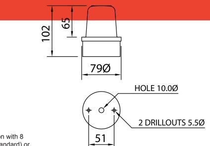
Multi-function Rotating/Pulsed/Static LED Beacon with 8 operating modes. Comprising a robust White (standard) or Black (option) ABS Base, and a Polycarbonate lens.
