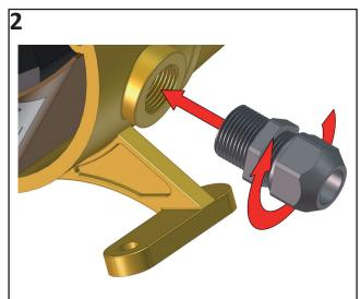
Whilst a cable gland is supplied, it is the installer's responsibility that it is both fitted correctly and suitable for the supply cable in use.
