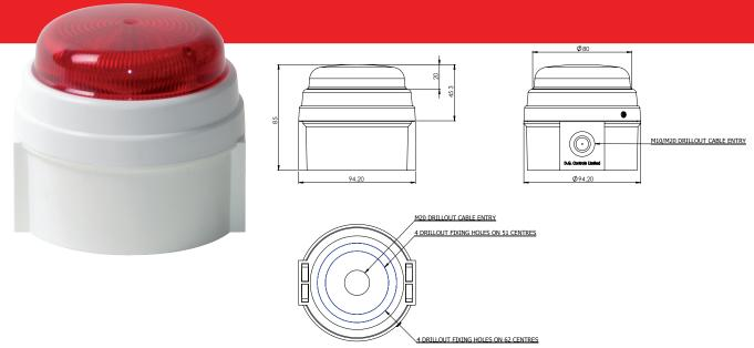
PSC - Pulsed (Flashing) LED warning beacons with internal jumper to select Static (Continuous) option.
